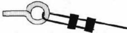
Two cable crimps or clamps must be used on each cable end. Cover the free ends of the cable with a crimp or tape to prevent pokes from the sharp wires.
